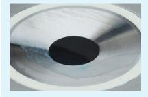
An improperly cleaned prism, where sample residue is left in the measurement well, can mix with a water zero or calibration fluid. This type of contamination during the calibration process will cause an error across all subsequent measurements.
